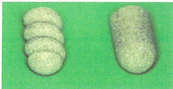
Fig 1 The two experimental plasma-sprayed-hydroxyapatite (PS-HA) designs used in this study. The implant on the left has a grooved surface, while the implant on the right has a smooth cylindrical design with a rounded apex. The occlusal surfaces (not visible) are not coated with HA ceramic.
